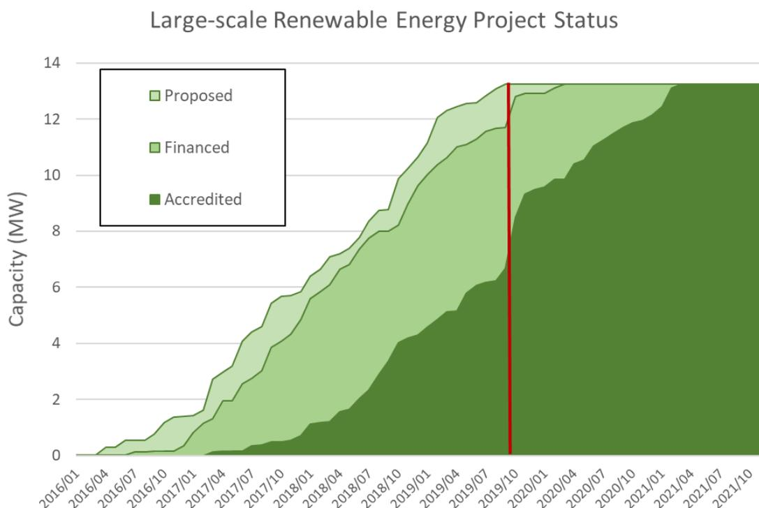
Figure 1. Status of large-scale renewable energy installations in Australia. Data to the right of the red line are forecasts based on publicly announced projects. For comparison, Australia’s average and peak demand for electricity is 24 and 36 GW respectively.
